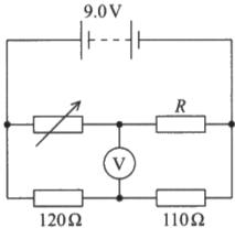
As the student adjusted the variable resistor, the reading on the voltmeter changed. When the variable resistor had a resistance of  $295 \Omega$ , the reading on the voltmeter was 0V. This happened because the p.d. across the variable resistor was equal to the p.d. across the  $120\Omega$  resistor.
