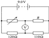
As the student adjusted the variable resistor, the reading on the voltmeter changed. When the variable resistor had a resistance of  $295 \Omega$ , the reading on the voltmeter was 0V. This happened because the p.d. across the variable resistor was equal to the p.d. across the  $120 \Omega$  resistor.
