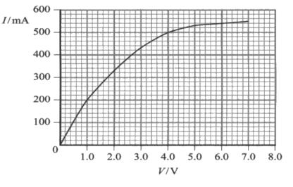
This filament lamp is connected across a battery of e.m.f. 6.0V as shown below.
