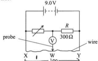
(i) The student moved the probe attached to the voltmeter along the wire until, at W, the reading on the voltmeter was 0V. This occurred when the length XW was 33.0 cm.
