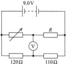
As the student adjusted the variable resistor, the reading on the voltmeter changed. When the variable resistor had a resistance of  $295\Omega$ , the reading on the voltmeter was <u>0V</u>. This happened because the p.d. across the variable resistor was equal to the p.d. across the 120 $\Omega$  resistor.
