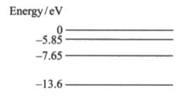
An electron in the atom is excited to the -5.85 eV energy level. The electron then makes the transition to the -7.65 eV energy level.
