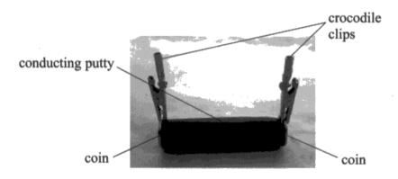
(a) The student made a cylinder of conducting putty of length 0.075 m and diameter 9.0 mm. Calculate the resistance of the cylinder of conducting putty.
