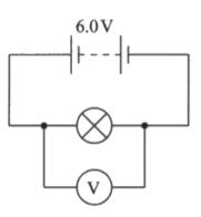
The voltmeter reading is 4.2 V.
