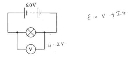
The voltmeter reading is 4.2 V.
